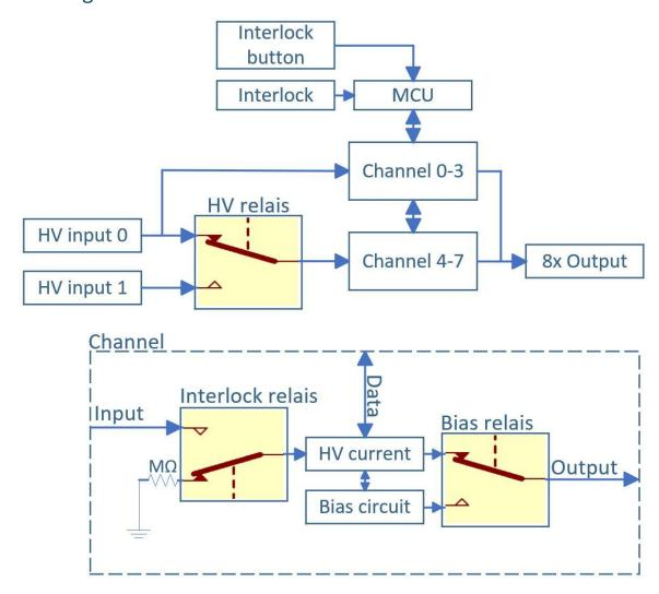
Note: the HV relays is now the switch in the front and not an uC-controlled relays
