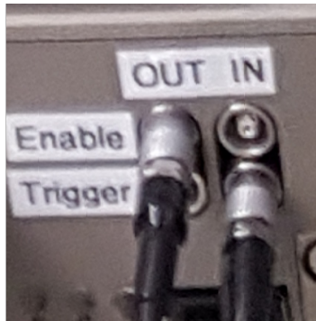
Figure 5: Trigger INPUT (looking at a single module from the back, top) is the rightmost, down .
