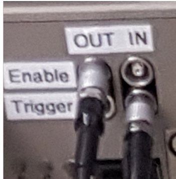
Figure 4: Trigger INPUT (looking at a single module from the back, top) is the rightmost, down .
