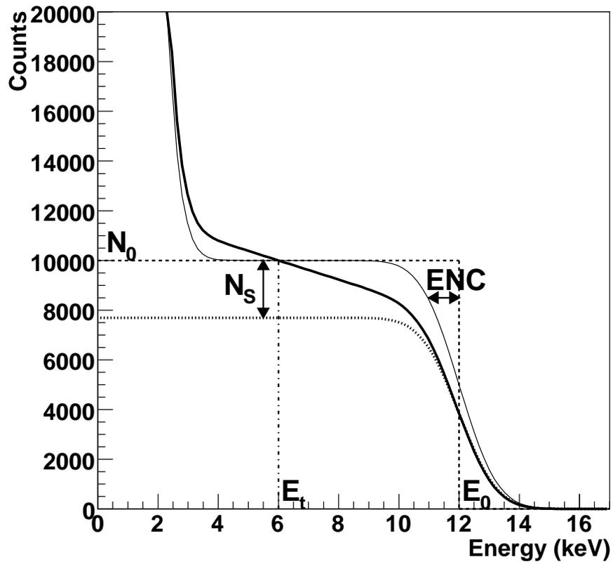
Figure 2: Measured threshold scan at 12.5 keV with the three different settings. In the inset the fit of the experimental data with the expected curve as in function 1 is shown in the region of the inflection point.
