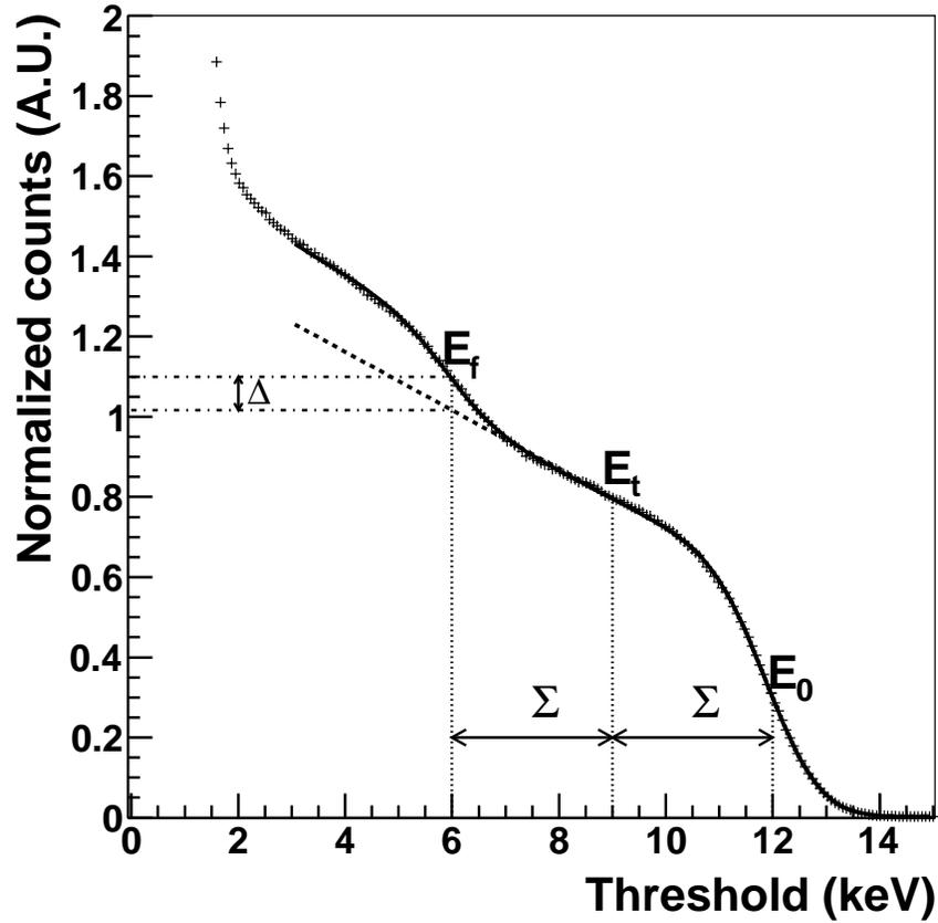
Figure 4: Median of the number of counts as a function of the threshold for X-rays of 12.5, 17.5 and 25 keV for one of the detector modules using *standard* settings. The solid line represents the fit of the experimental points with equation 1. In the inset the linear fit between the X-ray energy and the position of the inflection point of the curves is shown.
