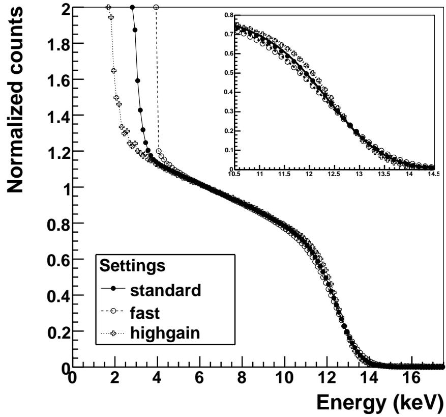
Figure 3: Number of counts as a function of the threshold measured from a sample containing iron ( $E_f=5.9$  keV) when using X-rays of energy  $E_0=12$  keV. In this case, setting the threshold at  $E_0/2$ , which is very close to  $E_f$ , would give  $\Delta \sim 10\%$  counts from the fluorescence background. Therefore the threshold should be set at an intermediate level  $E_t$  between the two energy components with a distance of at least  $\Sigma > 3ENC$  from both  $E_f$  and  $E_0$ .
