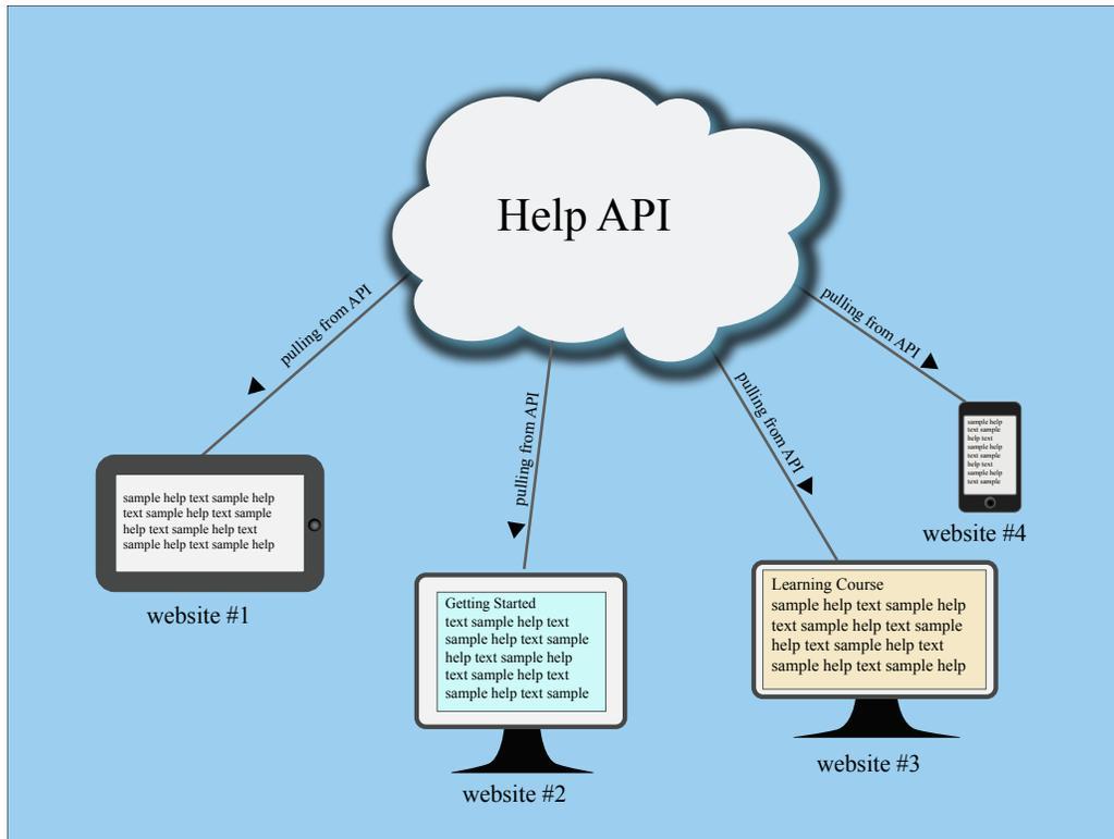
Is this really an API? Well, sort of. The help content is pushed out into a JSON file that other websites and applications can easily consume. The endpoints don't deliver different data based on parameters added to a URL. But the overall concept is similar to an API: you have a client requesting resources from a server.
